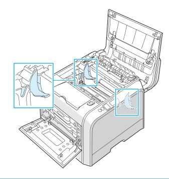
**CAUTION**: To prevent damage, do not expose the imaging unit to light for more than a few minutes. Close the top and left cover should the setup need to be halted for any reason.
